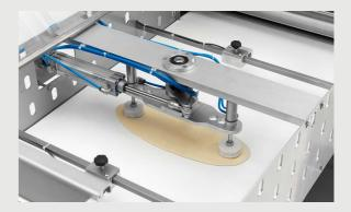
Rotation of the pizza with manipulator to reduce the overall dimensions of the machine in the laboratory
