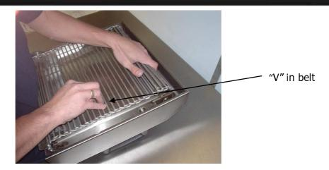
6 The open link of the belt can be un-hooked once the belt has been held down.
