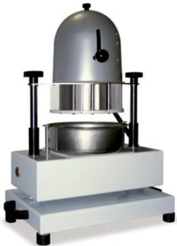
**UK** This is a compact and fully manual machine. The tank can hold up to 4.2 kg of pizza dough. The divider includes a cutting unit with 14 divisions. This makes it possible to always obtain 14 portions between 70 g and 300 g. The manually operated shaft moves the cutting unit down towards the bowl, which divides the dough. It is an easy to use machine that permits high hourly production rates. The portion tolerance is a few grams.
