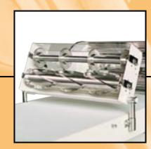
Cutting roller for use with the SF600 model.
