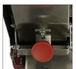
Blade adjustment handle To set the height and depth of the cut in the bread.
